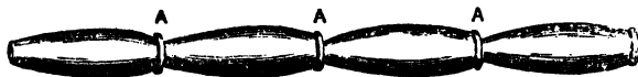
Fig. 73. Mode of arranging the Aludels or Adopters, at Almaden , for the condensation of the mercurial vapour. At \Delta \Delta \Delta the joints are closed with a clay lute.
